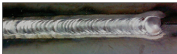
► Wave Bead of Aluminum
